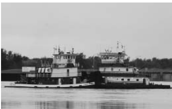
The M/V Paddy Cenac and the M/V Severn work together to clear shoaling problems at the lock forebay
