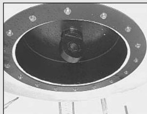
There is no extension beneath the buoy to puncture barges if the buoy capsizes
