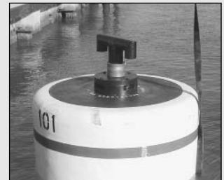
The t-head design prevents lines from "rolling free" of the buoy
